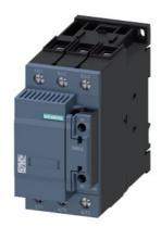
Capacitor contactor, AC-6b 75 kVAr, / 400 V 1 NO + 1 NC, 230 V AC, 50/60 Hz 3-pole, Size S2 screw terminal
