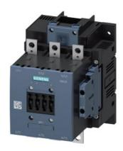
power contactor, AC-3 185 A, 90 kW / 400 V AC (50-60 Hz) / DC operation 110-127 V AC/DC auxiliary contacts 2 NO + 2 NC 3-pole, frame size S6 busbar connections drive: conventional screw terminal
