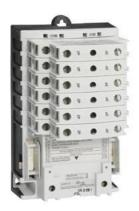
Electrically held lighting contactor, (convertible to mech. held), Amp rating 30A (tungsten 20A), 3 N.C. / 5 N.O. poles, 200-208V 60Hz coil, Noncombination type, Enclosure NEMA type (open), No enclosure
