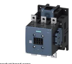
power contactor, AC-3 225 A, 110 kW / 400 V AC (50-60 Hz) / DC operation 440-480 V AC/DC auxiliary contacts 2 NO + 2 NC 3-pole, frame size S10 busbar connections drive: conventional screw terminal
