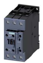
Power contactor, AC-3 80 A, 37 kW / 400 V 1 NO + 1 NC, 42 V AC, 50 Hz 3-pole, size S2 screw terminals
