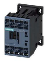
Power contactor, AC-3 7 A, 3 kW / 400 V 1 NO, 24 V DC 0.8-1.1\*Us with integrated varistor, 3-pole, Size S00, Spring-type terminal
