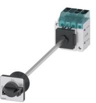
Load disconnector 3LD3, lu 25 A Main switch 3-pole + N Rated operating capacity at AC-23 A at 400V 9.0kW floor mounting Basic switch with door coupling Central hole mounting 22.5mm Toggle drive black 48x48 mm with auxiliary switch 10E + 1S
