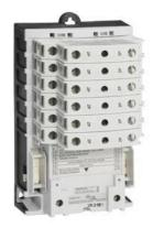
Electrically held lighting contactor, (convertible to mech. held), Amp rating 30A (tungsten 20A), 7 N.C. / 1 N.O. poles, 277V 60Hz / 240V 50Hz coil, Non-combination type, Enclosure NEMA type (open), No enclosure
