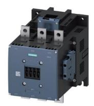
power contactor, AC-3 500 A, 250 kW / 400 V AC (50-60 Hz) / DC 96-127 V AC/DC auxiliary contacts 2 NO + 2 NC 3-pole, frame size S12 busbar connections drive: electronic with PLC interface 24 V DC screw terminal
