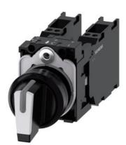
Selector switch, illuminable, 22 mm, round, plastic, white, selector switch, short, 3 switch positions I>O<II, momentary contact type, 10:30h/12h/13:30h, with holder, 2x1NO+1NC, Spring-type terminal
