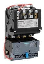
Non-reversing motor starter Size 0 Three phase full voltage Solid-state overload relay OLRelay amp range 0.75-3.4A 240VAC 50HZ / 277VAC 60HZ coil Combination type No enclosure
