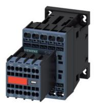
Power contactor, AC-3 9 A, 4 kW / 400 V 2 NO + 2 NC, 230 V AC 50/60 Hz, 3-pole, Size S00 Spring type terminal Captive auxiliary switch
