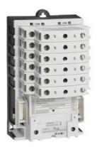
Electrically held lighting contactor, (convertible to mech. held), Amp rating 30A (tungsten 20A), 2 N.C. / 4 N.O. poles, 230-240V 60Hz/220V 50Hz coil, Non-combination type, Enclosure NEMA type (open), No enclosure
