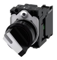
Selector switch, illuminable, 22 mm, round, plastic, white, selector switch, short, 2 switch positions O-I, latching, 10:30h/13:30h, with holder, 1 NO, screw terminal, with laser labeling, upper case
