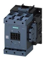
power contactor, AC-3 185 A, 90 kW / 400 V AC (50-60 Hz) / DC operation 23-26 V AC/DC auxiliary contacts 2 NO + 2 NC 3-pole, frame size S6E busbar connections drive: conventional with 2 box terminals 3RT19 56-4G up to 120 mm
