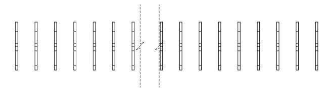
NOTE: CONTACTS ARE HELD IN A CARRIER FOR EASE OF ASSEMBLY
