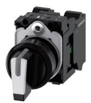
Selector switch, illuminable, 22 mm, round, plastic, white, selector switch, short, 3 switch positions I-O-II, latching, 10:30h/12h/13:30h, with holder, 1 NO, 1 NO, spring-type terminal, with laser labeling, inscription or symbol Customer-specific selection with SIRIUS ACT configurator (CIN)
