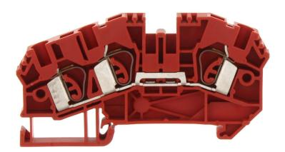
Feed-through terminal, Tension-spring connection, Mounting type: Mounting rail TS 35/7.5, Rated cross-section: 4 mm², Width: 6.1 mm, Colour: Red
