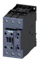
power contactor, AC-3 51 A, 22 kW / 400 V 1 NO + 1 NC, AC / DC 84-155 V, with varistor, 3-pole, size S2, screw terminal
