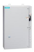
Non-reversing motor starter, Size 0, Three phase full voltage, Solid-state overload relay, OLR amp range 3-12A, Combination type, 10A circuit breaker, Enclosure NEMA type 4/12, Water/dust tight for outdoors, Extrawide enclosure
