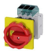
Load disconnector 3LD3, lu 16 A Main switch 3-pole Rated operating capacity at AC-23 A at 400V 7.5kW Front plate mounting Basic switch with Central hole mounting 22.5mm Rotary actuator red / yellow 66 x 66 mm with auxiliary switch 1OE + 1S
