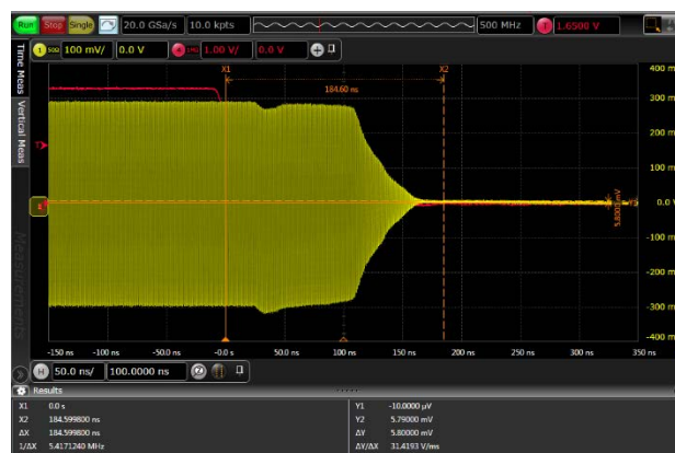
Figure 16. Switching Time Insertion Loss to Isolation State
