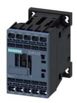
Coupling contactor relay railway 4 NO, 110 V DC, 0.7 ... 1.25\* US, with integrated varistor, Size S00, Spring-type terminal
