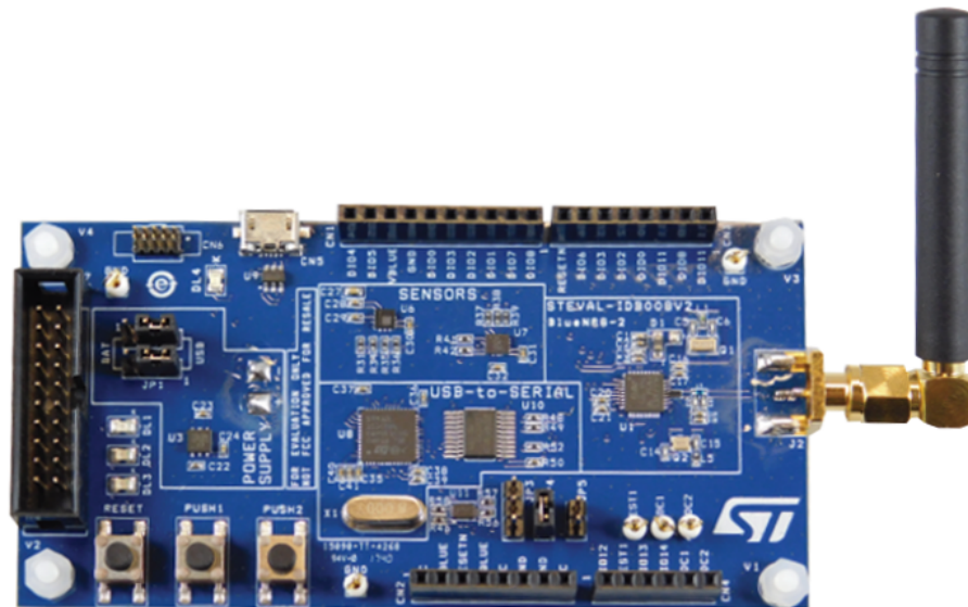
Figure 4. STEVAL-IDB008V2 development platform
