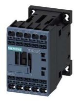
Power contactor, AC-3 7 A, 3 kW / 400 V 1 NC, 24 V DC, 0.8-1.1\*Us with integrated varistor, Size S00, Spring-type terminal
