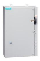
Non-reversing motor starter, Size 2, Three phase full voltage, Solid-state overload relay, OLR amp range 13-52A, 24VAC 50-60Hz coil, Combination type, 50A circuit breaker, Encl NEMA type 4X 316 S-Steel, Water/dust tight noncorrosive, Extra-wide enclosure
