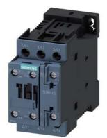
power contactor, AC-3 17 A, 7.5 kW / 400 V 1 NO + 1 NC, AC (50-60 Hz) DC operation 21-28 V AC/DC, 3-pole, Size S0, screw terminal
