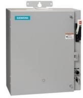
Pump control panel, Size 3, Three phase full voltage, Solid-state overload relay, OLR amp range 25-100A, 190-220/220-240V 50/60Hz coil, Standard type contactor, 200A fusible disconnect, 200A/600V fuse clip, HOA Sel Sw. <(>&<)> Start P.B., Enclosure NEMA type 3/3R, Weather proof outdoor use
