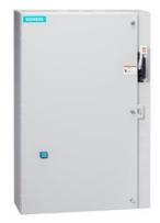
Non-reversing motor starter, Size 4, Three phase full voltage, Solid-state overload relay, OLR amp range 50-200A, Combination type, 200A non-fusible disconnect, Enclosure NEMA type 1, Indoor general purpose use, Standard width enclosure
