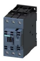
Traction contactor, AC-3 65 A, 30 kW / 400 V 1 NO + 1 NC 24 V DC, 0.7-1.25  $^{\circ}$  Us with varistor 3-pole, size S2 Spring-type terminals
