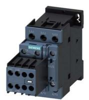
power contactor, AC-3 9 A, 4 kW / 400 V 2 NO + 2 NC, 220 V AC 50 / 60 Hz, 3-pole, Size S0, screw terminal Removable auxiliary switch
