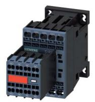
contactor relay, 6 NO + 2 NC, 220 V AC 50 Hz 240 V 60 Hz, size S00, spring-loaded terminal, captive auxiliary switch
