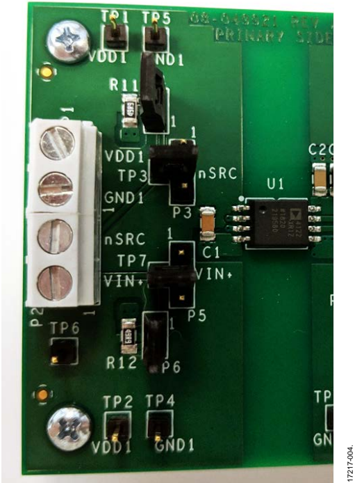
Figure 4. P3 and P5 Configured for Screw Terminal Input
