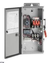
Slim Line Pump Control Panel NEMA size 1 Three phase full voltage Solidstate overload relay OLR amp range 10-40A 110/120V 50/60Hz Coil 30A fusible disconnect 30A/250V fuse clip 1NC / 1NO auxiliary contacts HOA Sel. Sw. <(>&<)> Start/Stop 3-point power terminal block 3-point control terminal block 3-point ground lug Enclosure NEMA type 3/3R Weather proof outdoor use
