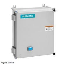
Non-reversing motor starter, Size 3 1/2, Three phase full voltage, Solidstate overload relay, OLR amp range 50-200A, 110V 50Hz / 120V 60Hz coil, Non-combination type, Enclosure type 4X fiberglass, Water/dust tight noncorrosive, Standard width enclosure
