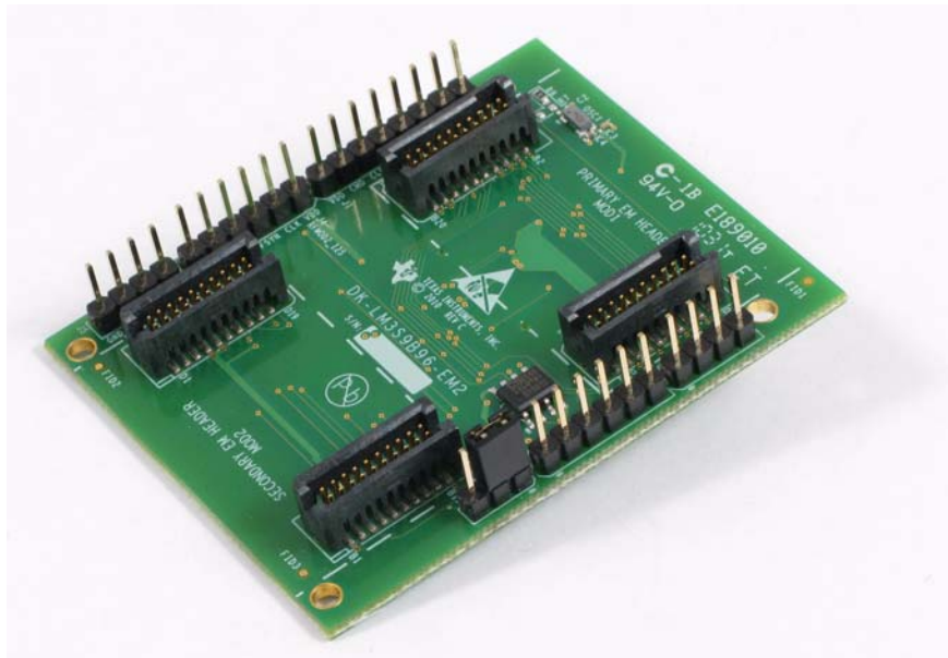
Figure G-1. EM2 Expansion Board
