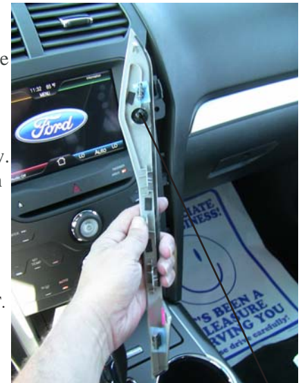
Bezel removal (plastic lug)
