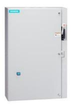
Non-reversing motor starter Size 4 Three phase full voltage Solid-state overload relay OLRelay amp range 50-200A 110-120/220-240VAC 60HZ coil Combination type 150A circuit breaker Enclosure NEMA type 1 Indoor general purpose use Standard width enclosure
