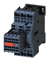
Contactor, AC-3, 15 kW / 400 V, 2 NO + 2 NC, 110 V AC, 50 Hz, 120 V, 60 Hz, with inserted varistor, 3-pole, Size S0 Spring type terminal Captive auxiliary switch
