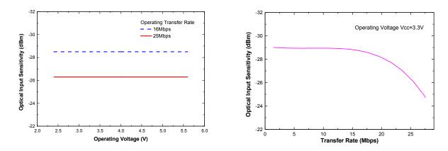
**Note:** Before using the PLR233 series device, please confirm the minimum sensitivity at different operating voltage and transmission rate.
