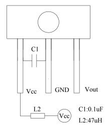
Note: 1. For having good coupling, the C1 capacitor must be placed within 7mm
