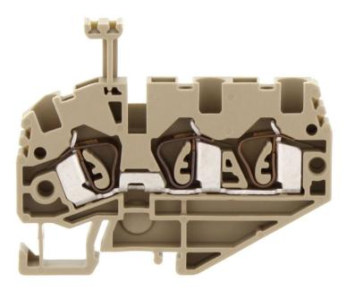
Feed-through terminal, Tension-spring connection, Mounting type: Mounting rail TS 15/5.5, Rated cross-section: 2.5 mm<sup>2</sup>, Width: 5.1 mm, Colour: Yellow
