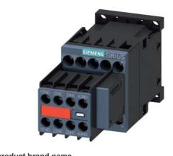
Power contactor, AC-3 7 A, 3 kW / 400 V 2 NO + 2 NC, 230 V AC 50 / 60 Hz, with varistor plugged on, 3-pole, Size S00 Screw terminal Captive auxiliary switch block
