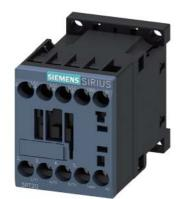
Power contactor, AC-3 7 A, 3 kW / 400 V 1 NO, 480 V AC, 60 Hz 3-pole, Size S00 screw terminal
