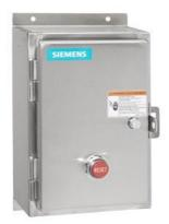
Non-reversing motor starter, Size 3 1/2, Three phase full voltage, Amb. compensate bimetal OLR, Contactor amp rating 115A, 24VAC 50-60Hz coil, Non-combination type, Encl. type 4X 304 S. Steel, Water/dust tight noncorrosive
