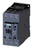
Power contactor, AC-3 80 A, 37 kW / 400 V 1 NO + 1 NC, 208 V AC 50/60 Hz, 3-pole Size S2, screw terminals
