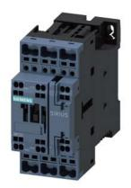
Traction contactor, AC-3 25 A, 11 kW / 400 V 1 NO + 1 NC with electronic drive 72 V DC, 0.7-1.25\* US, with integrated varistor, 3-pole, Size S0, Spring-type terminal
