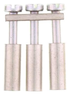
Cross-connector, No. of poles: 3, Mounting type: Can be screwed on, Width: 17 mm, Rated cross-section: 4 mm<sup>2</sup>, Colour: natural
