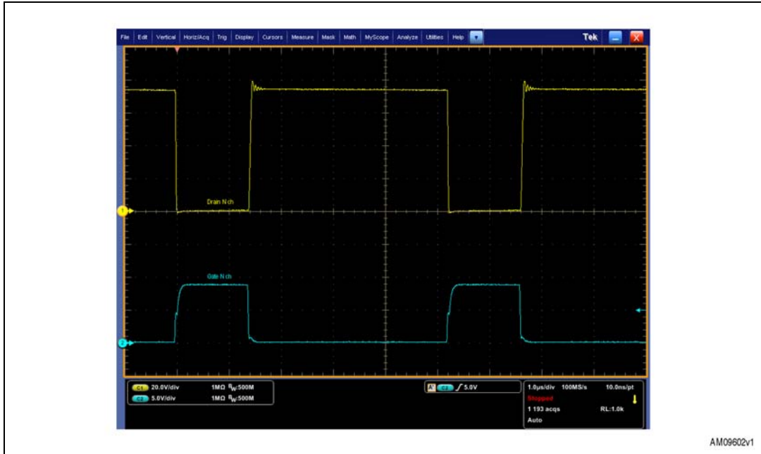
Figure 19. Primary side power MOSFET waveforms at 0 A load
