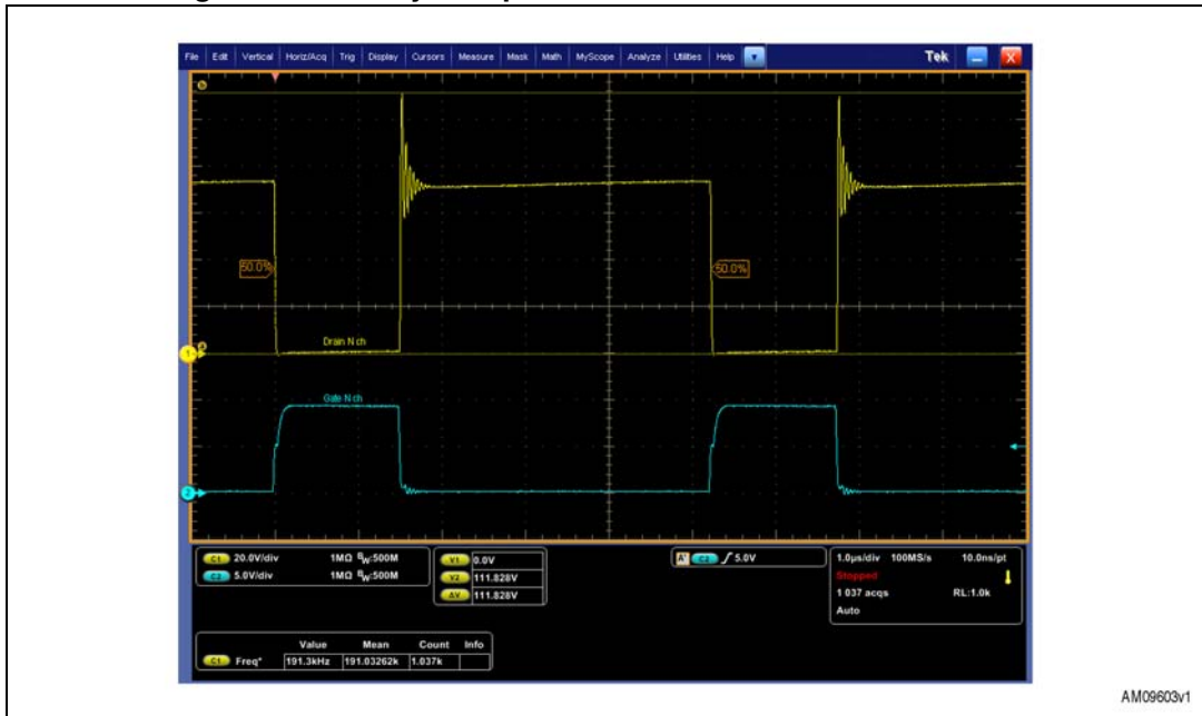
Figure 20. Primary side power MOSFET waveforms at 4 A load
