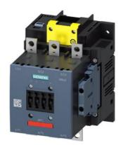
Power contactor, AC-3 115 A, 55 kW / 400 V Coil AC 50/60 Hz and DC 200-277 V x (0.8-1.1) F-SPS input 24 V DC 3-pole size S6 Auxiliary contacts 2 NO + 2 NC permanently mounted Main circuit: Busbar Control and auxiliary circuit: Screw terminal
