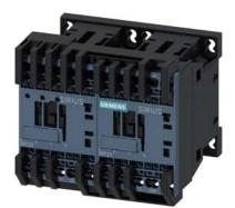
Reversing contactor assembly for 3RA27 AC-3, 3 kW/400 V, 24 V DC 3-pole, Size S00 Spring-type terminal electrical and mechanical interlock with voltage tap
